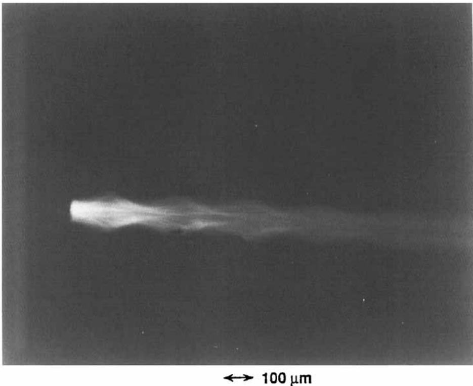
FIGURE 5 Propagation modes in nematic (E7) liquid-crystal cylindrical waveguide near the optical fiber input.
